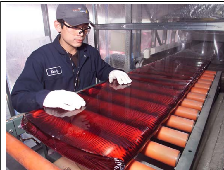
Figure 13.1 : Nd:doped phosphate laser glass coming off the production line of the continuous melt process developed for the NIF and LMJ laser systems.
