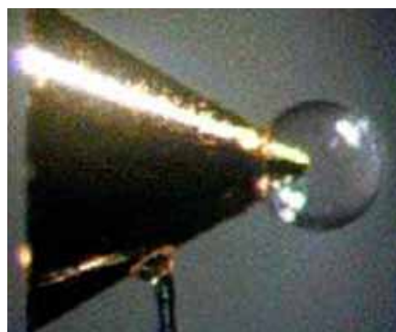
Glitter ball: Gold is used in the target pellet's core because of its malleable and smooth properties
